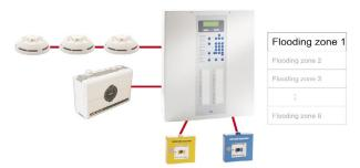
In the networked Extinguishing Control Panel LCnet216, up to 127 extinguishing systems with a total of 127 flooding zones can be implemented. Each extinguishing system can control up to 32 flooding zones, and each LCnet sectional control panel can administrate up to 8 flooding zones.
